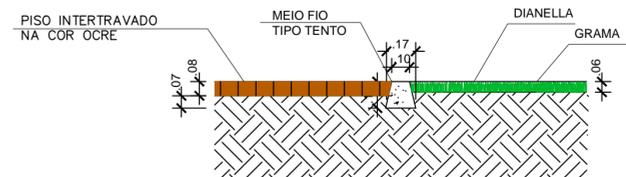
DETALHE PISO INTERTRAVADO X GRAMADO ESC 1/25
