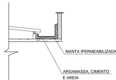
DETALHE CALHA ESC 1/75
