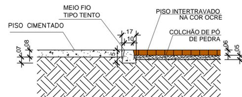
DETALHE PISO CIMENTADO X PISO INTERTRAVADO ESC 1/25
